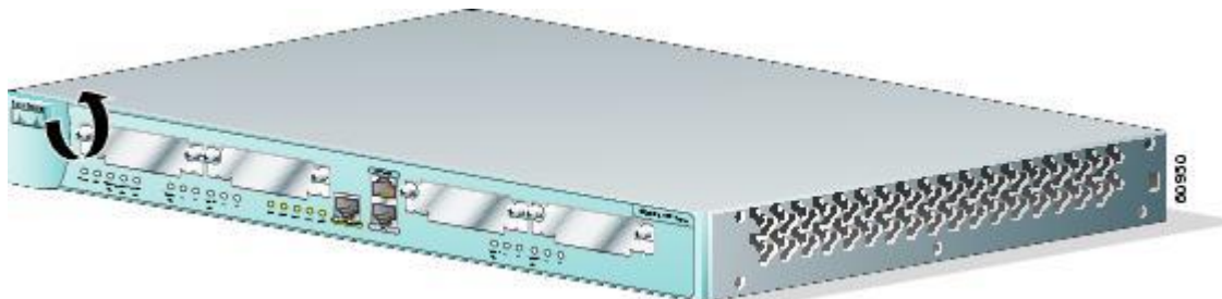
Figure 5 Removing a WIC or VIC Slot Cover
