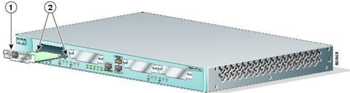
Figure 6 Inserting a WIC or VIC in the Router
